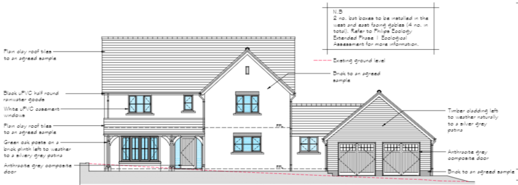
PROPOSED SOUTH WEST ELEVATION @ 1:100
